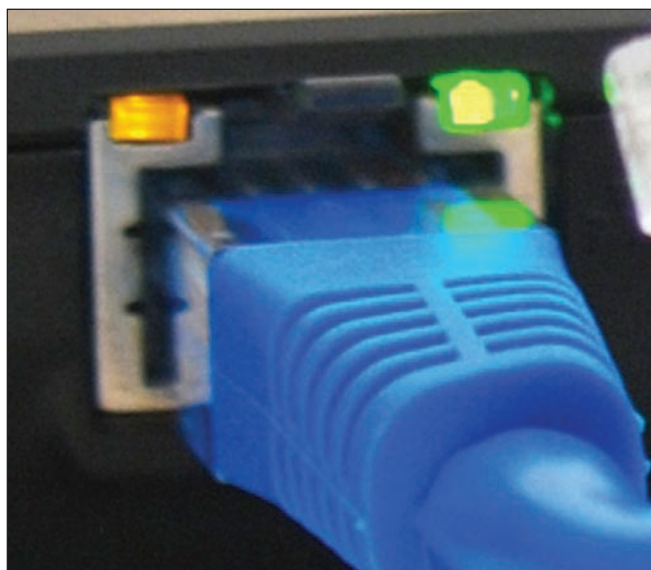
Figure 3-30 Status indicator lights for the onboard network port
