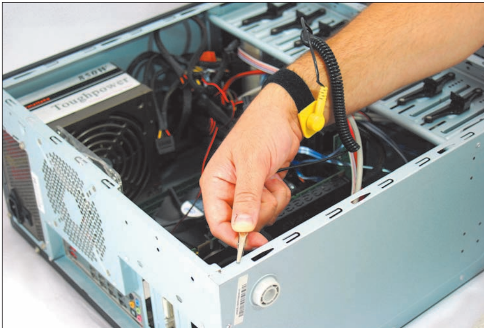
Figure A-7 A ground bracelet, which protects computer components from ESD, can clip to the side of the computer case and eliminate ESD between you and the case
