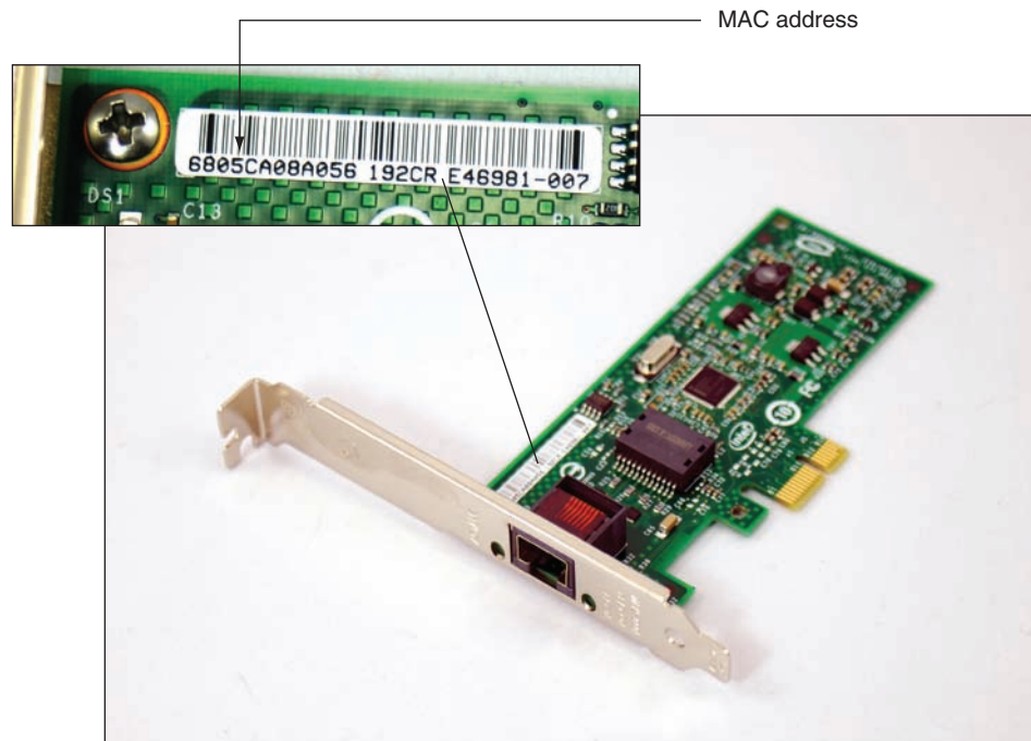
Figure 3-29 This Gigabit Ethernet adapter by Intel uses a PCIe ×1 slot
