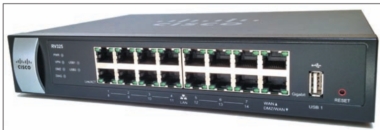
Figure 3-34 A router connects the local network to the Internet
