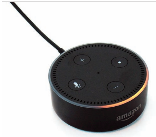
Figure 9-48 The orange light indicates the Echo Dot is on but not connected to a Wi-Fi network
