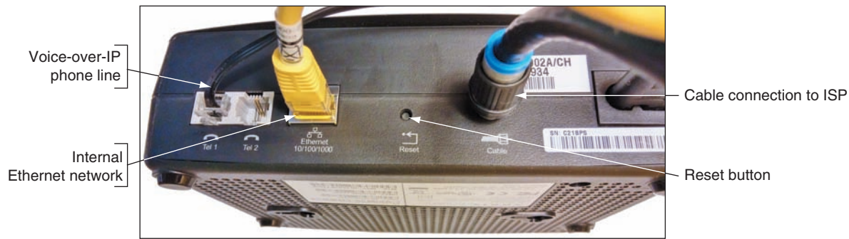
Figure 3-4 Use a cable modem to connect the ISP's coaxial cable to the LAN's Ethernet cable
