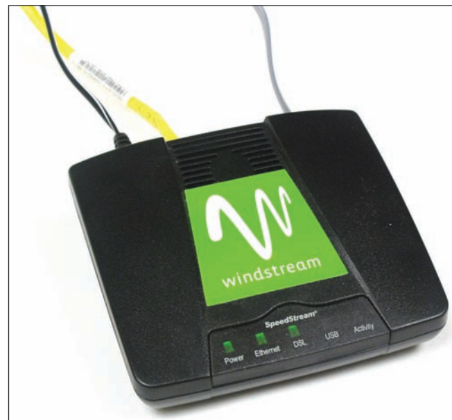
Figure 3-3 This DSL modem connects to a phone jack and a computer or router to provide a broadband connection to an ISP
