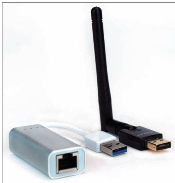
Figure 3-27 USB devices provide wired and wireless network connections
