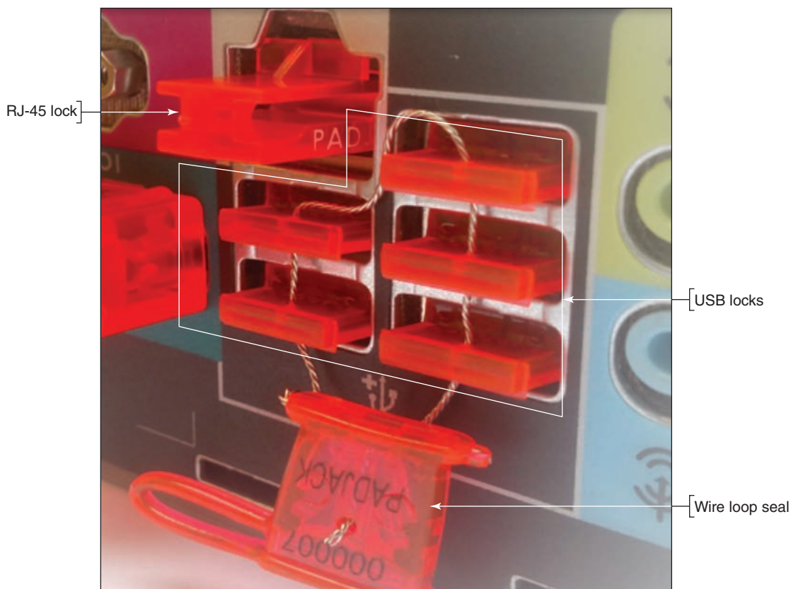
Figure 8-3 These port locks are reusable, but the wire loop seal can be used only once
