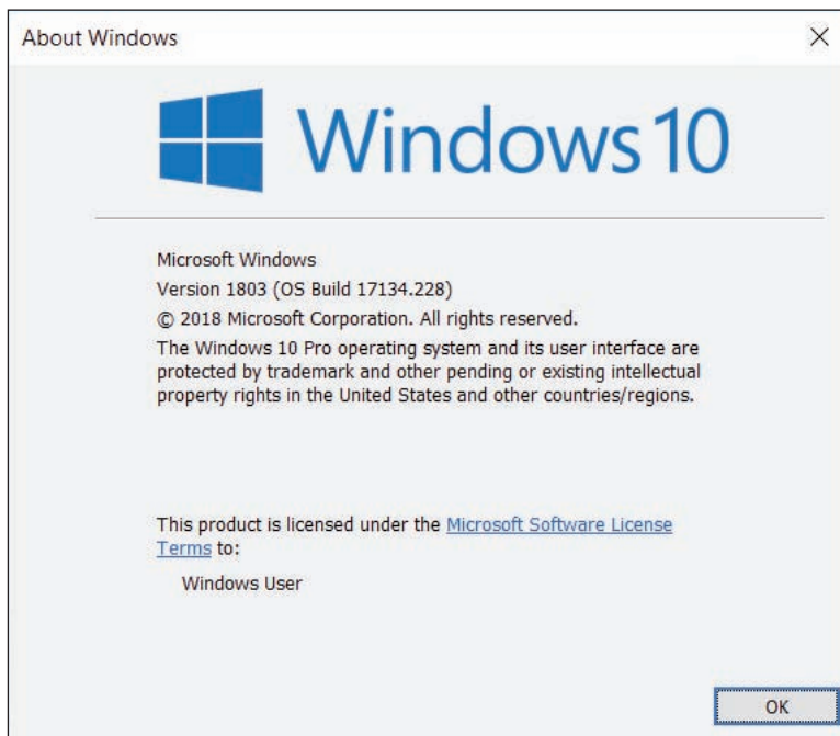
Figure 6-28 Version and build numbers can identify the major and minor Windows updates installed
