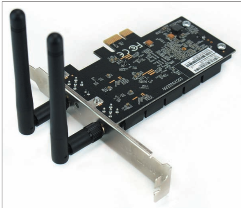
Figure 3-54 A wireless network adapter with two antennas supports 802.11a/b/g/n/ac Wi-Fi standards
