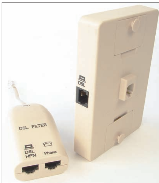
Figure 3-2 When DSL is used in your home, filters are needed on every phone jack except the one used by the DSL modem
