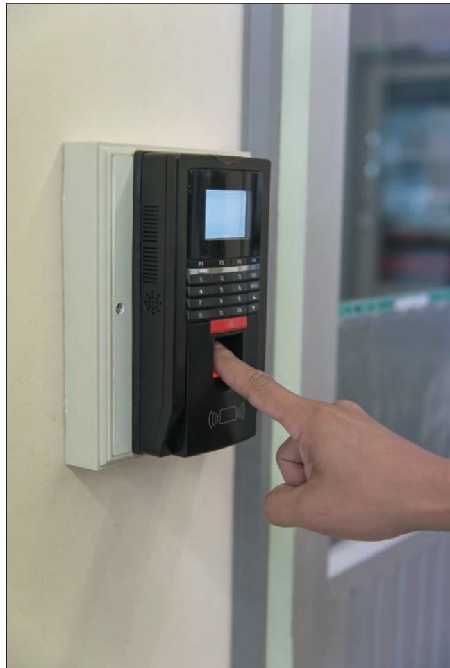
Figure 8-1 This access control device accepts typed code, fingerprint, or smart card input
