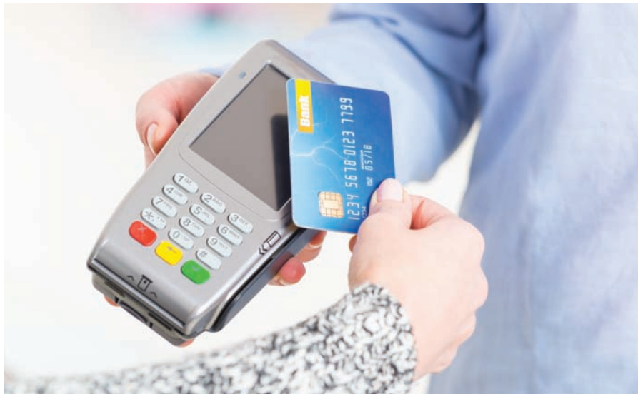
Figure 8-7 A smart card is read by a wireless smart card reader
