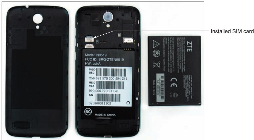
Figure 3-7 A SIM card contains proof that your device can use a cellular network
