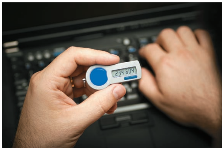
Figure 8-8 A security token such as this key fob is used to authenticate a user gaining access to a secured network
