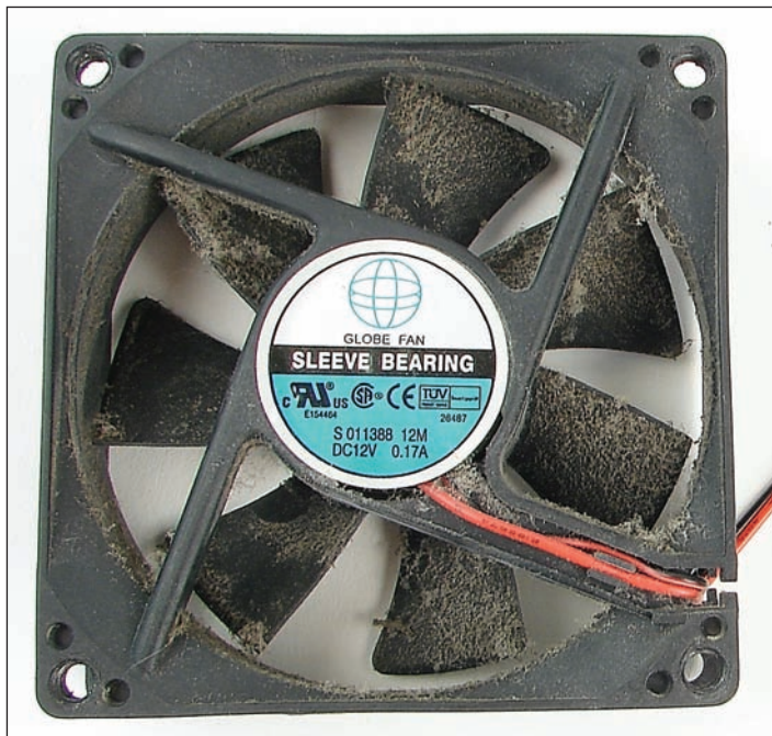
Figure A-12 This dust-jammed case fan caused a system to overheat
