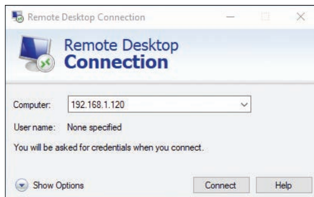
Figure 4-41 The IP address of the remote computer can be used to connect to it
